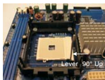
STEP 1: Lift Up The Socket Lever
